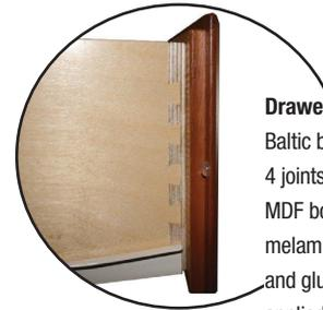
**Drawer boxes** consist of 1/2" 9-ply Baltic birch plywood dove-tailed on all 4 joints. The drawer bottom is a 1/4" MDF board with a white thermo-fused melamine, captured on all four sides and glued in place. Drawer fronts are applied separately.
