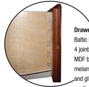
**Drawer boxes** consist of 1/2" 9-ply Baltic birch plywood dove-tailed on all 4 joints. The drawer bottom is a 1/4" MDF board with a white thermo-fused melamine, captured on all four sides and glued in place. Drawer fronts are applied separately.
