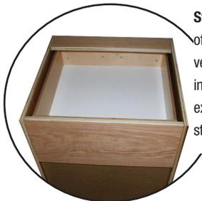
**Stretcher rail construction** consists of a horizontal front rail and two vertical back rails that are doweled into the cabinets ends...providing excellent structural rigidity and strength
