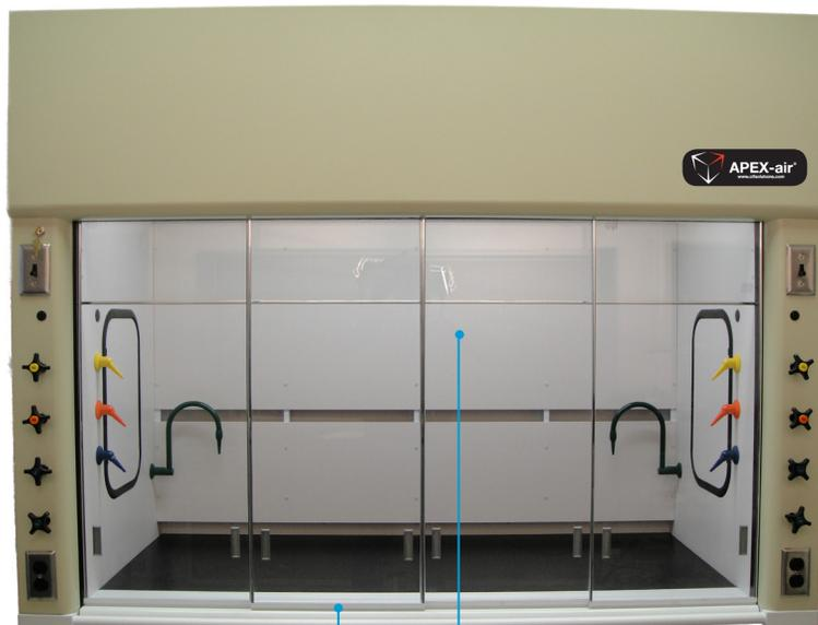
**SAFETY: Lower Sash Handle** is designed to be aerodynamic, eliminating turbulence as air enters the hood.
