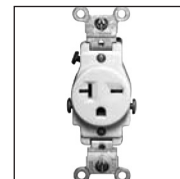
NEMA #6-20R single receptacle 250 VAC, 20 Amp
